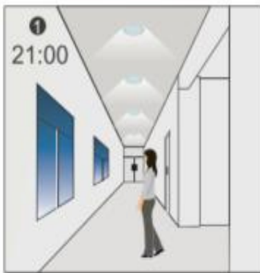
1 The Light Switches On At100% When There Is Movement Detected.
