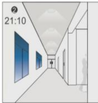
2 The Light Dims To Stand-by level After The Hold-time.
