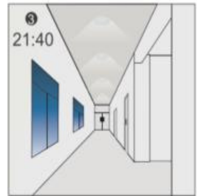
3 The Light Remains In Dimming Level At Night.
