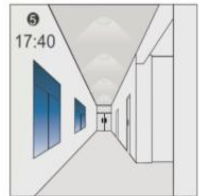
5 The Light Automatically Turnson At 10% When Natural Lightis Insufficient (no Motion).
